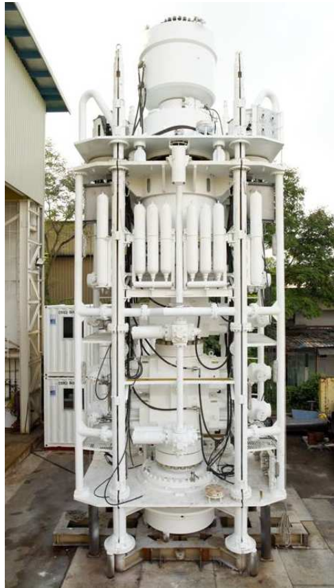
Rebuilt and complete stack-up 18 3/4" – 15,000 PSI Blowout Preventer for semi-submersible rig
